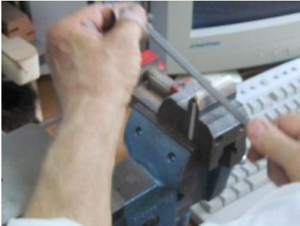
Filing the curve on the back of the nut (towards the tuning machines).
