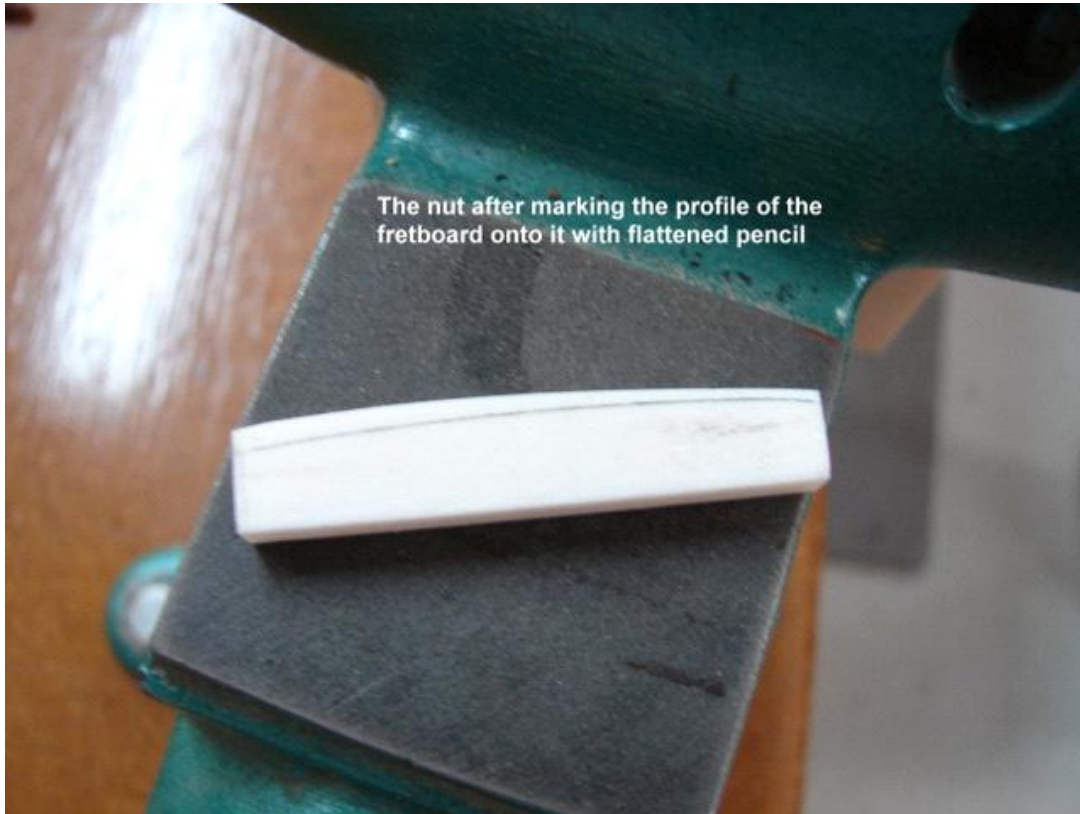
Nut after grinding. Notice the line.
