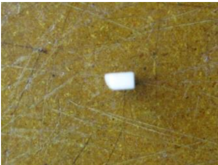
Resulting nut in profile. The ends are also domed to a hemispherical shape, much like the fret ends.
