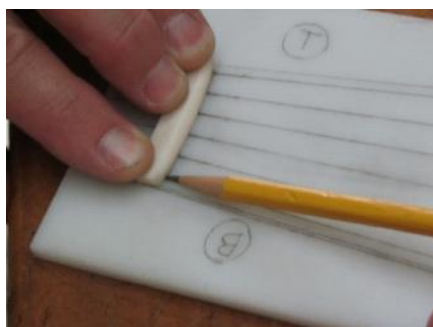
With a very sharp pencil, make a mark at each string location.
