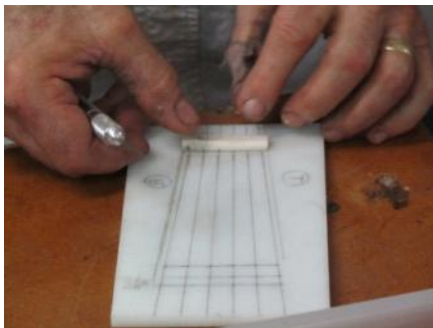
Laying out the nut slot locations. This template works for any nut width. String positions are not centered on the middle of the string. Rather, the space between string edges is equalized. Also, the template adds some extra bias to the bass side, as the 6th string is so much larger than the 1st. This is barely visible in the photo as a line on the bass side just outside the line that is symmetrical with the treble side.
